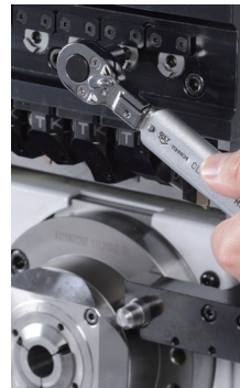
Tighten with a torque wrench
